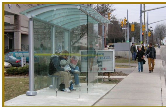
Locate transit shelters behind the Pedestrian Clearway
