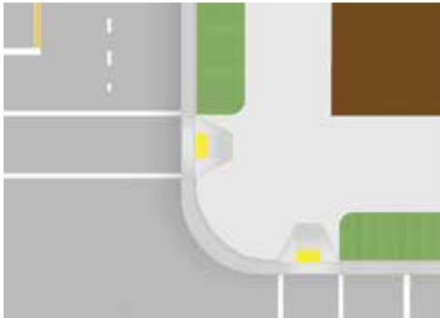
Figure 3.2-9: Appropriate ramp placement
