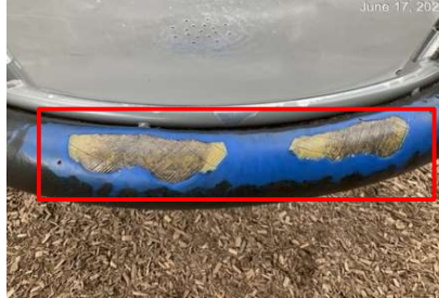
#11 - Area 3 - Saucer swing seats are wearing (exterior rubber)
